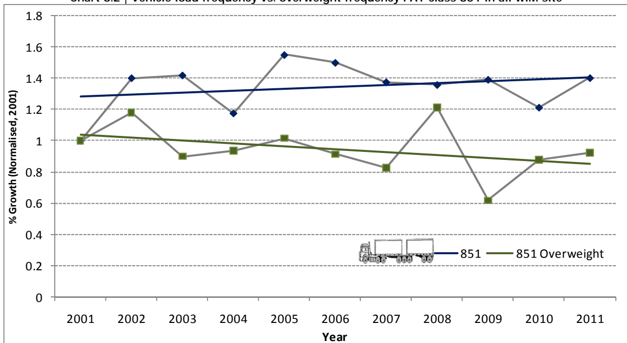
Chart 8.2 | Vehicle load frequency vs. overweight frequency PAT class 851 in all WiM site
