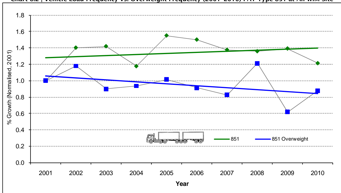
Chart 8.2 | Vehicle Load Frequency vs. Overweight Frequency (2001-2010) PAT Type 851 at All WiM Site
