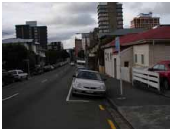
No stopping line marked over a driveway
