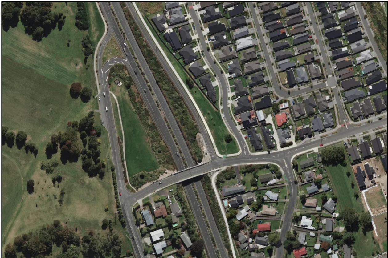
Figure 7-2: Grade separated intersection with on ramps and / or off ramps (Image source: LINZ)
