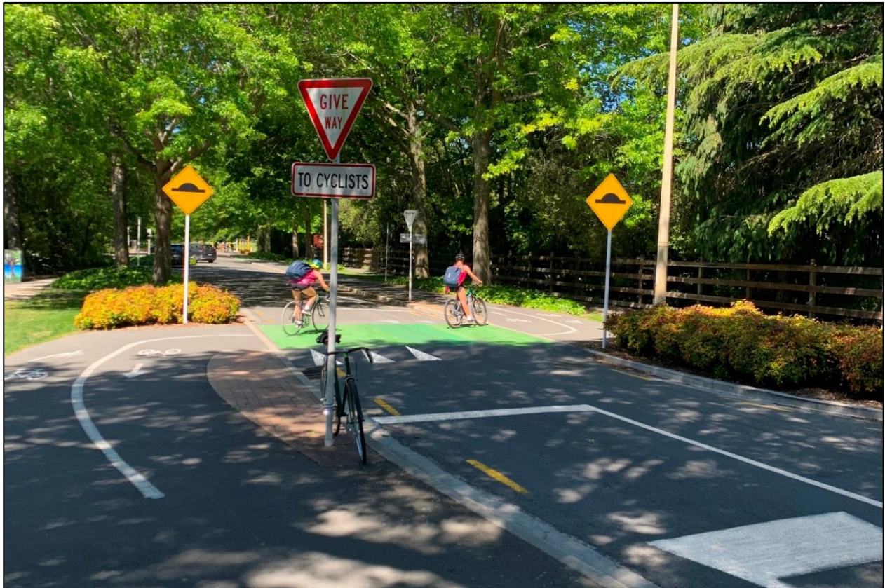
Figure 2-7: Intersection of a cycle path with a roadway, Matai Street East, Christchurch
