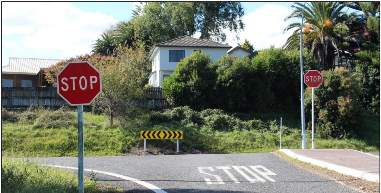
Figure 4-3: Example of Chevron sight board at T-intersection, black on yellow (W20-1.4) at head of intersection
