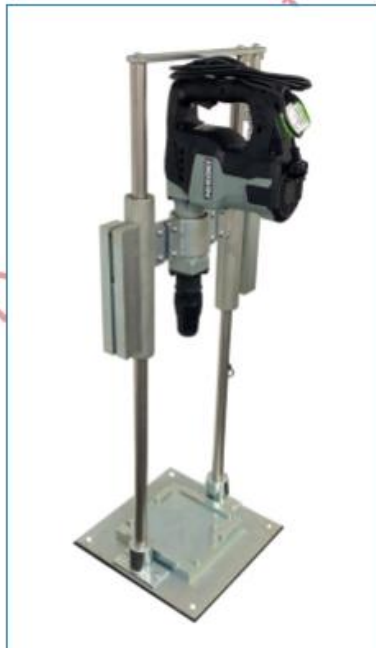
Figure 2: Vibrating Hammer and Loading Frame
