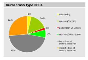
As shown above, nearly half of the rural crashes involved a vehicle losing control on a bend. While one third of these crashes occurred on a wet road, there was only one caused by an icy surface last year.
