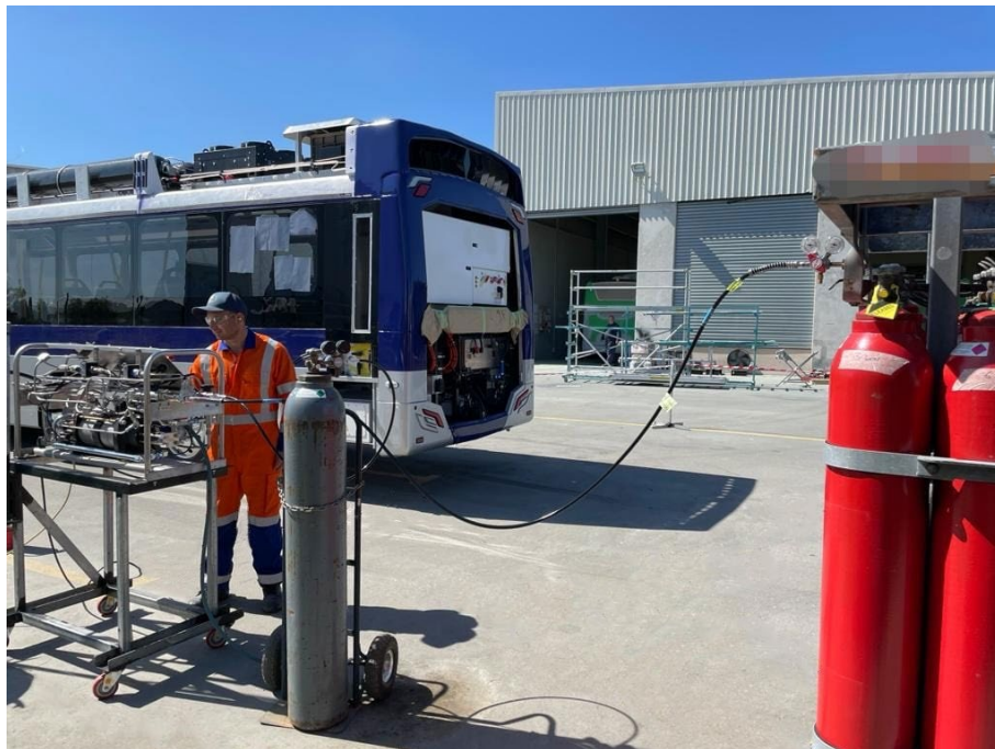
Figure 3.2 Interim hydrogen fuelling for Auckland's trial (Source: Bus & Coach Association)
