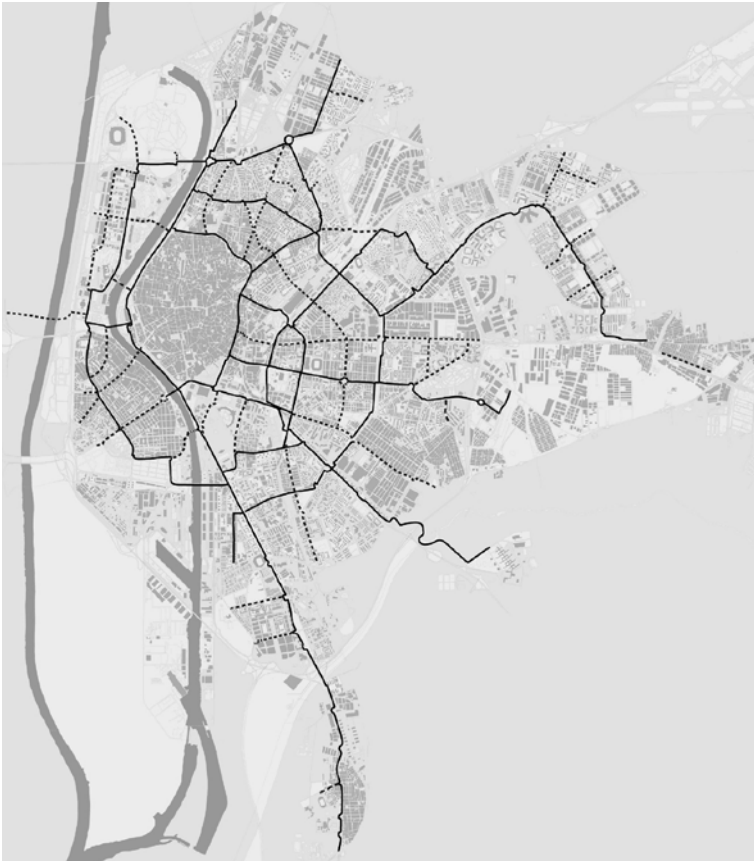
Figure 9.5 120 km cycle network developed in Seville, Spain, between 2006 and 2010 (Source: Marques et al., 2015, figure 1)
