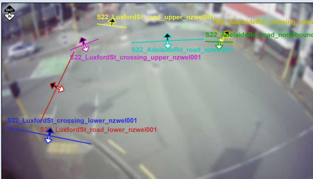
Figure 5-5 A single sensor in Wellington counts traffic across multiple links (reprinted from Wellington City Council, personal communication, 2024)
