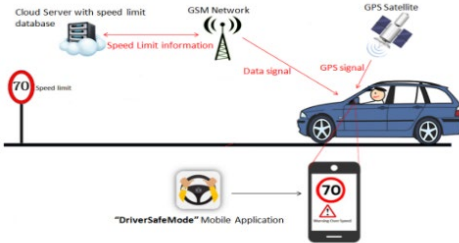
Figure 2.5. How the DriverSafeMode app works (reprinted from Perera & Dias, 2017, p. 341)
