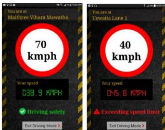
Figure 2.4 Visual of when complying with the speed limit (left) and warning when exceeding the speed limit (right) (reprinted from Perera & Dias, 2017, p. 340)
