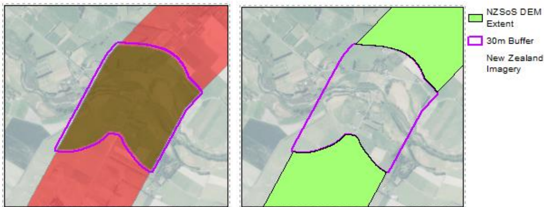
Figure 4.21 The brown area shows the extent of LIDAR coverage for this section of the corridor. The purple line shows a 30 m buffer region of this extent. This buffer region is then used to erase those areas of LIDAR coverage from the corridor which leaves only those areas requiring data from the lower resolution DEM (NZSoS DEM)
