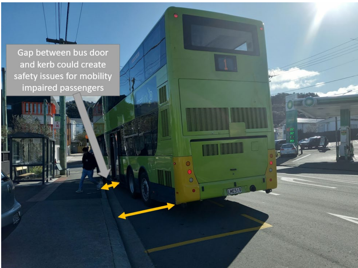
Figure 7.16 Gap created at the bus rear door
