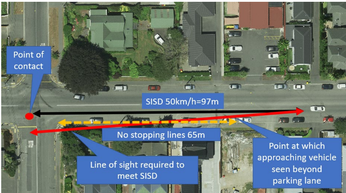
Figure 7.17 Sight distance requirements versus actual no-stopping restriction
