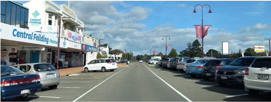
Figure 6.4 Angle parking on the side (60 degree) and the middle of the road (60 degree) (Fielding)
