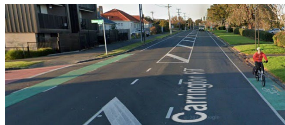
Figure 8.25: Existing cycle lanes next to kerb
