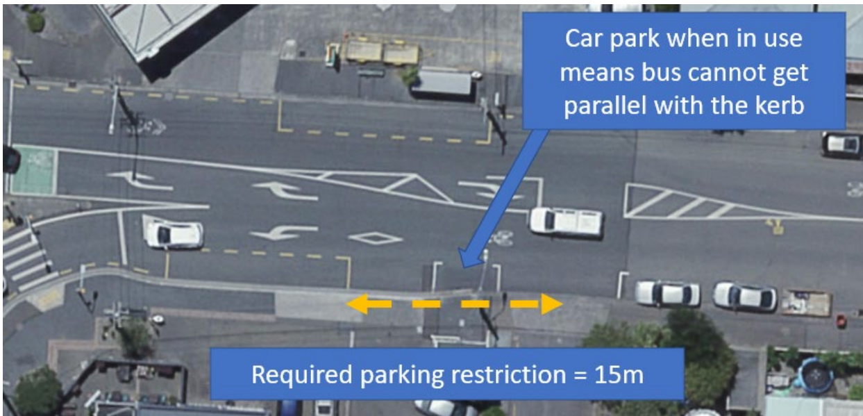
Figure 7.15 Parking restricts ability for bus for pull in parallel with the kerb
