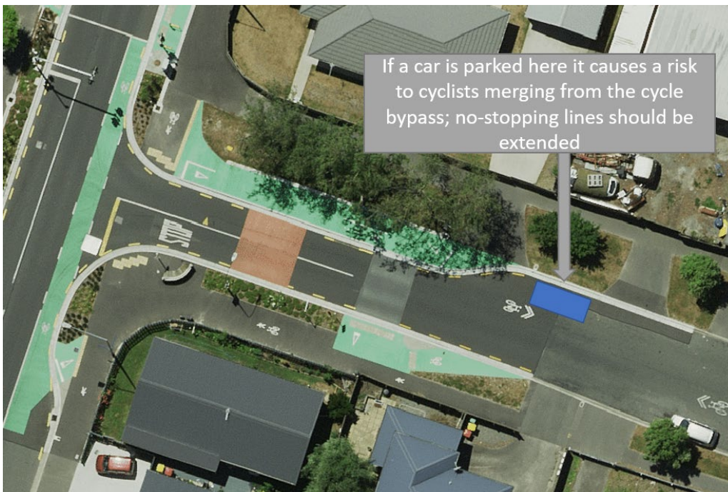
Figure 7.7 Parking restriction extends at cycle bypasses
