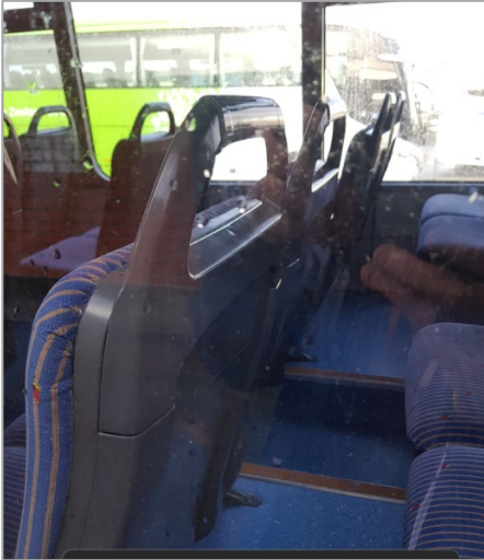
Figure 6.11 Example of hard plastic-backed seats on a New Zealand school bus (truck bus)
