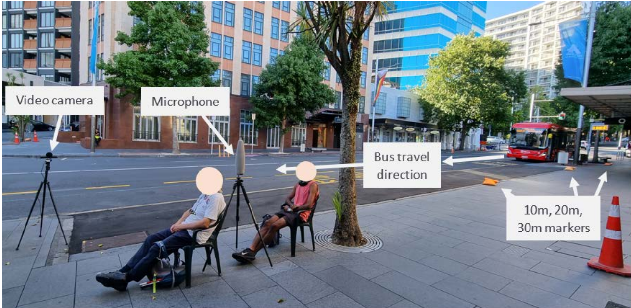
Figure 3.5 On-street testing set-up, Auckland
