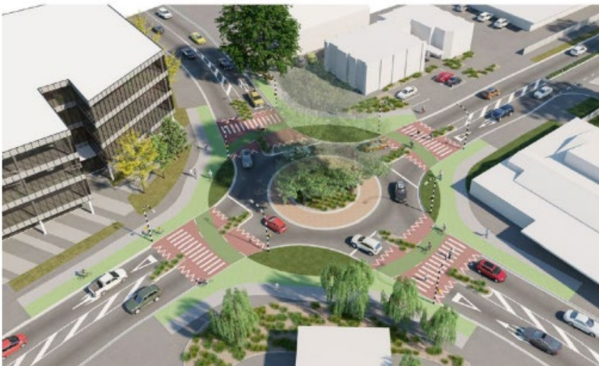
Figure 4.1 Dutch-style upgrade option for the Tristram Street/Collingwood Street roundabout (reprinted from Barton, 2021, p. 61)
