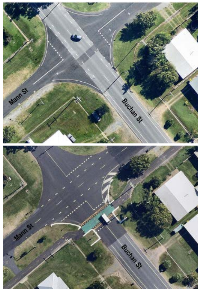
Figure 2.5 Before (top) and after (bottom) the introduction of a pathway, showing the path and intersection priority path for people who ride and walk (reprinted from Munro, 2018, p. 17)
