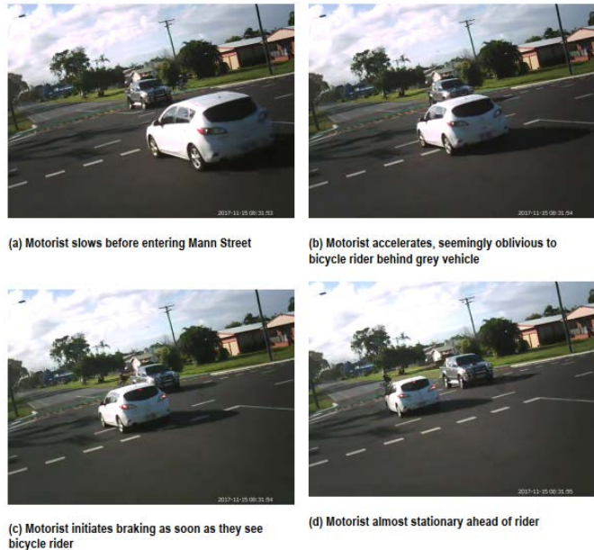
Figure 2.7 Example of an unintended outcome that can be observed via video-based methods, where a waiting vehicle ‘screened’ or reduced the visibility of a path user (reprinted from Munro, 2018, p. 23)
