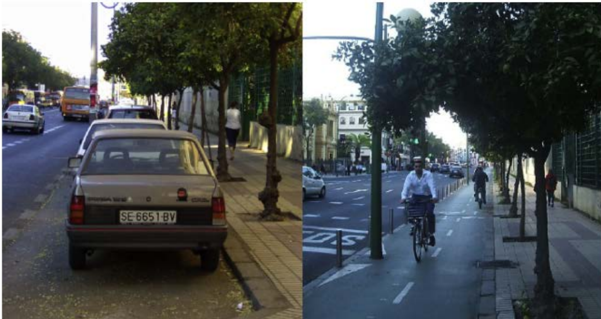
Figure 3.6 Example of before and after replacement of car parks with bi-directional cycleway in Seville, Spain (reprinted from Marqués et al., 2015, p. 35)
