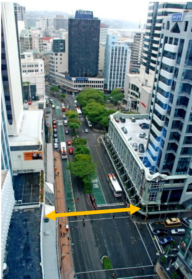
Figure 1.1 Lambton Quay, Wellington, with an arrow indicating the definition of a road as 'building-to-building'
