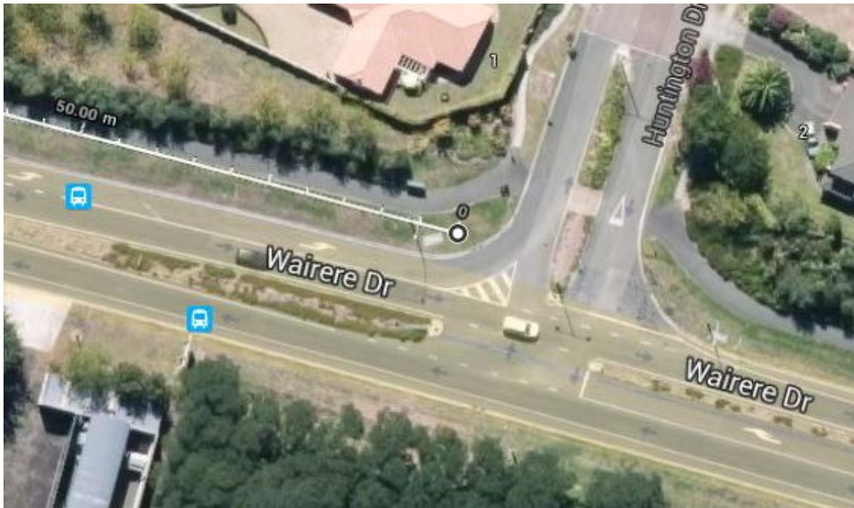
Figure 3 8 Priority T-intersection with room to wait in centre but small area for storage
