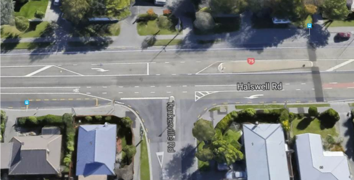
Figure 3.6 Priority T-intersection where right turn out is unlikely to be made in two steps
