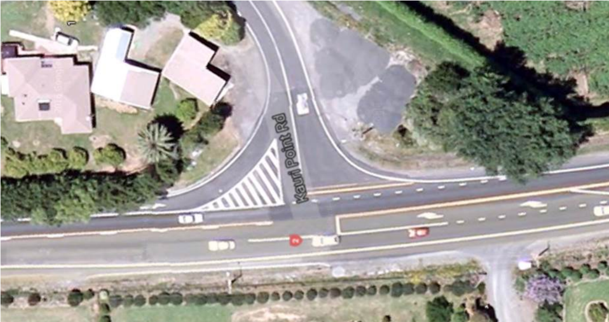
Figure 3.7 Priority T-intersection layout, where some aggressive drivers may use median space
