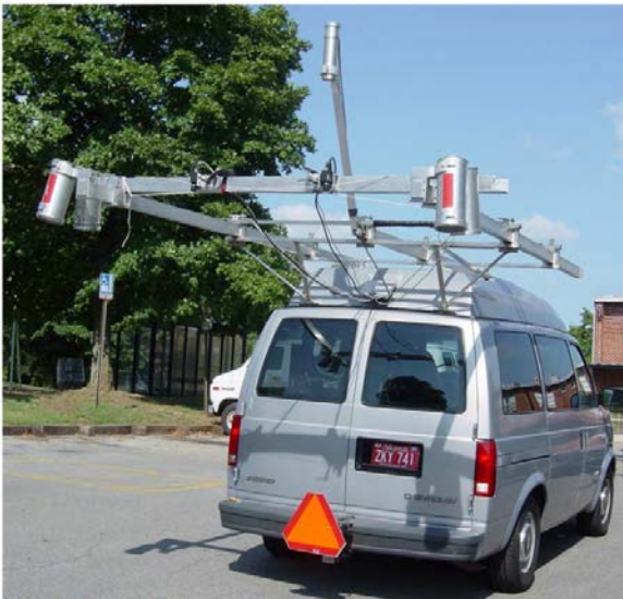
Figure 2.1 Digital data collection vehicle (Wang 2004)
