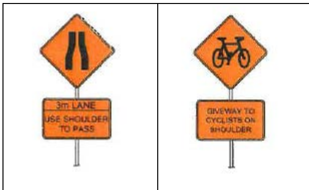
Figure 2.18 Treatment signage used to inform drivers of the upcoming 2- 1 design
