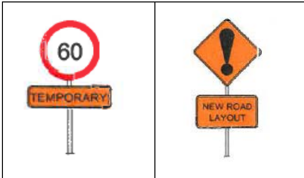
Figure 2.19 Treatment signage used to inform drivers of the upcoming 2- 1 design
