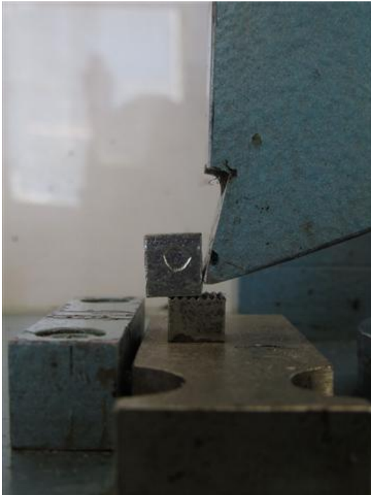
Figure 4.2 Vialit test specimen holder showing the point of impact by the pendulum
