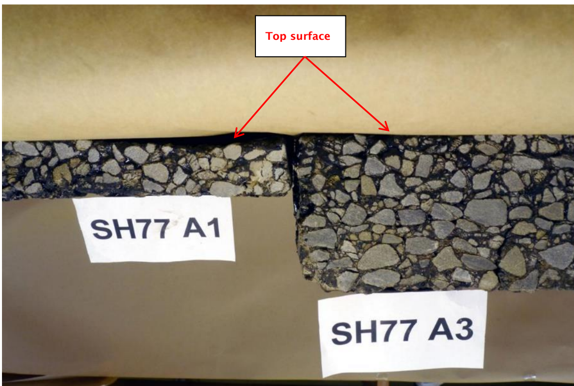
Figure 2.45 Site 3, comparison of intact specimen thickness (illustrating extent of loss due to stripping)
