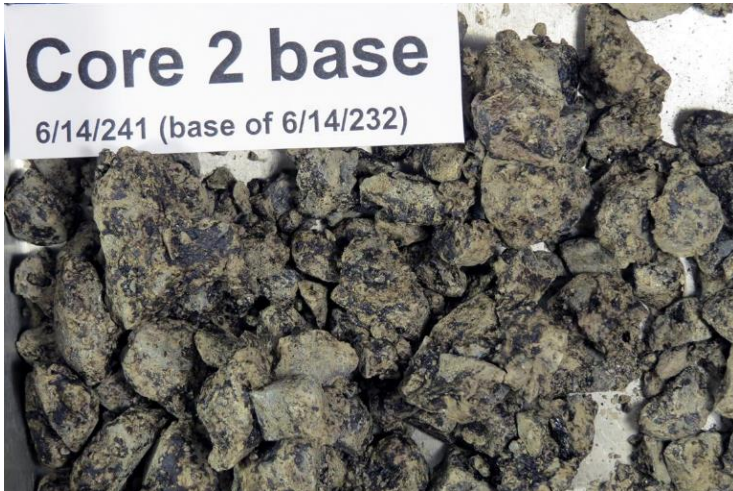
Figure 2.32 Site1, stripped, loose aggregate recovered from the base of core hole 2
