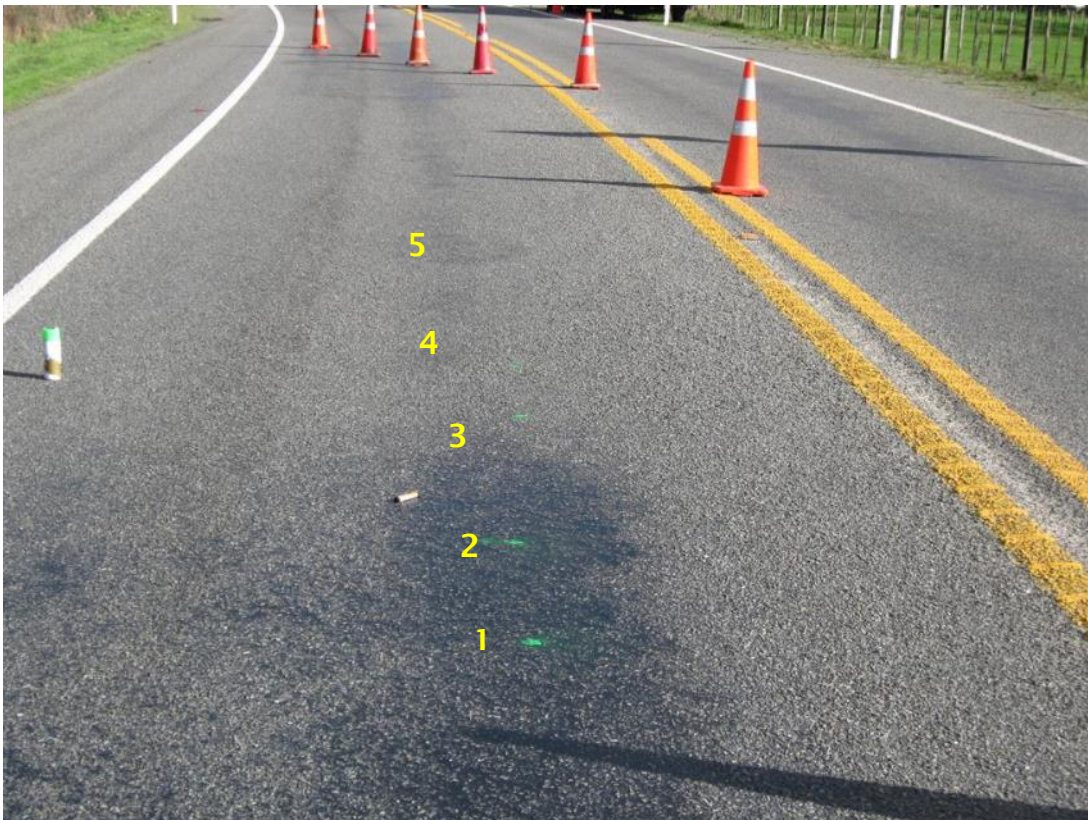
Figure 2.63 Site 7, showing the core positions
