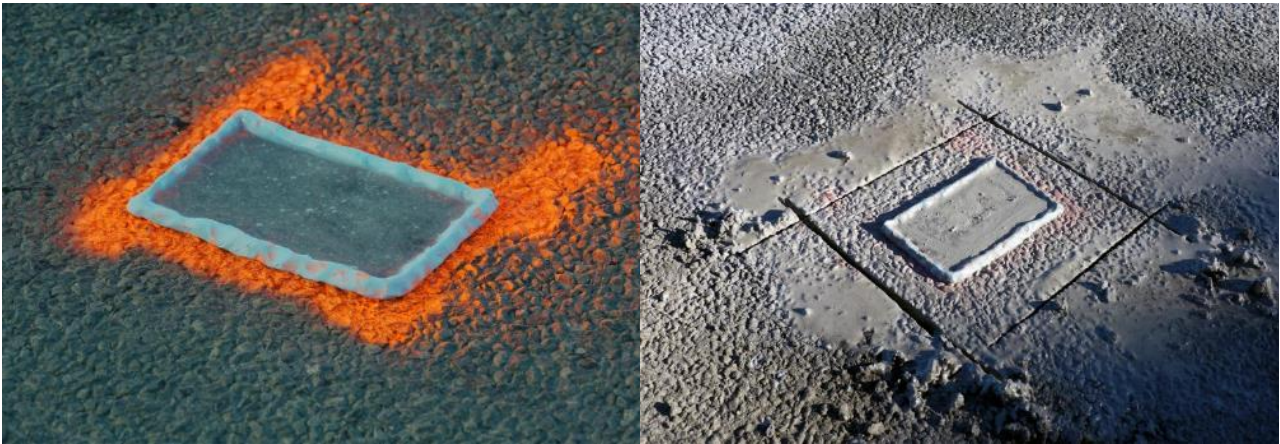
Figure 2.70 Method to examine first- coat seal basecourse embedment. Left, securing the chip with an epoxy resin. Right, cutting around the specimen that can now be removed without distorting the sample patch
