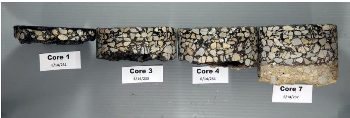
Figure 2.31 Site 1 cores showing a progression of seal loss through stripping. Core 1 (flushed) to core 7 (well textured)
