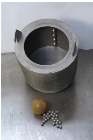
Figure 2.13 OMD test drum. The four metal protrusions on the inside of the drum catch the steel balls and aggregate and allow them to drop to the bottom of the drum increasing the amount of breakdown
