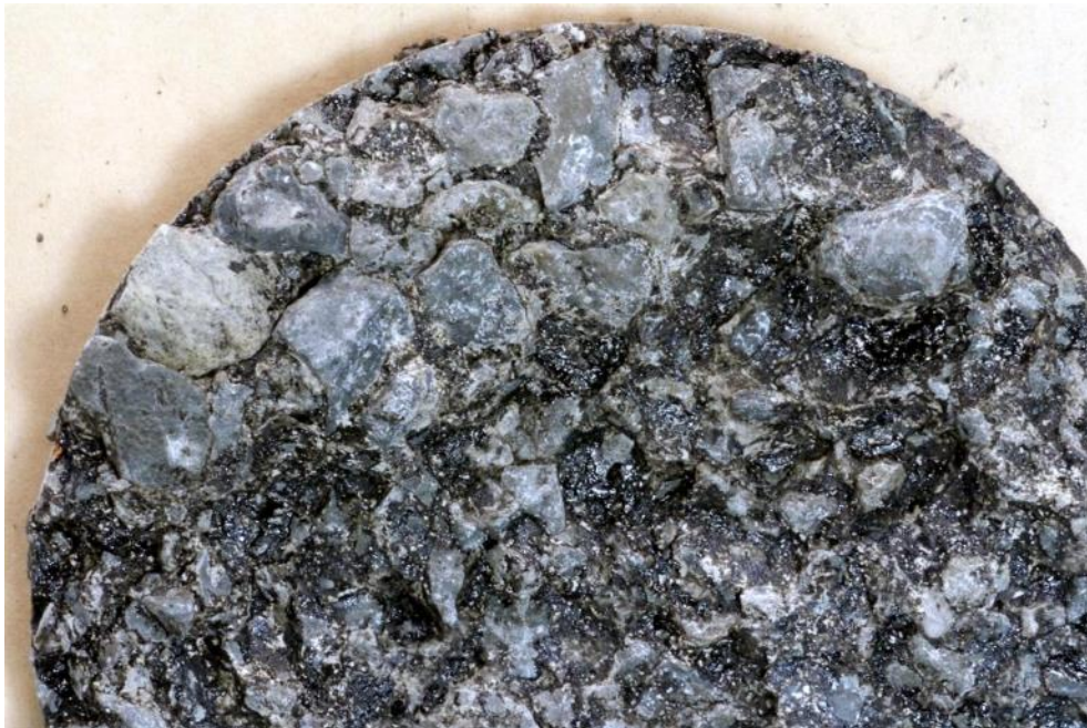
Figure 2.58 Site 5, base of specimen (core 9) from flushed patch showing stripped seal
