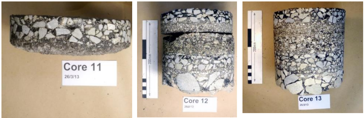
Figure 2.62 Site 6, cores 11, 12 and 13 showing the progression of stripping damage from the heavily flushed patch (core 11) to good seal texture (core 13)
