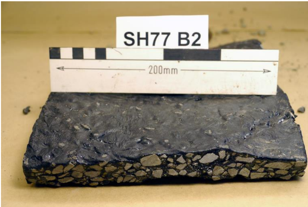
Figure 2.49 Site 4, specimen taken adjacent to the flushed patch
