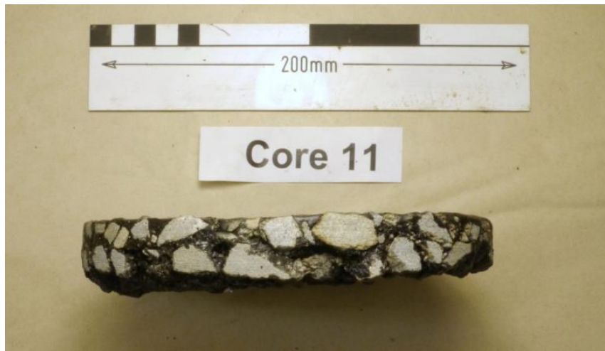
Figure 2.39 Site 2, close up of core 11 cross section from a flushed patch, manually broken to reveal the internal structure and evidence (deposited basecourse fines) for water migration through the layer
