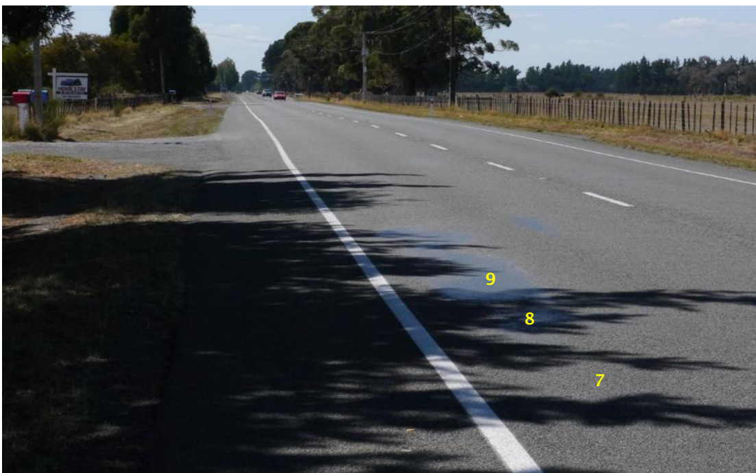
Figure 2.53 Site 5, flushed patch and core locations
