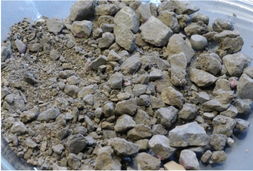
Figure 2.4 Example of aggregate breakdown material from a multi-layer chipseal core constructed from grade 2, 3 and 5 chip only
