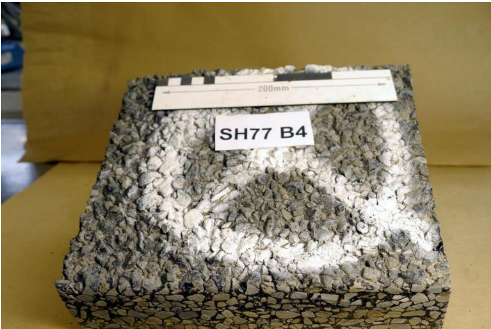
Figure 2.49 Site 4, specimen taken adjacent to the flushed patch
