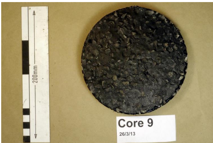
Figure 2.56 Site 5, top surface specimen from flushed patch
