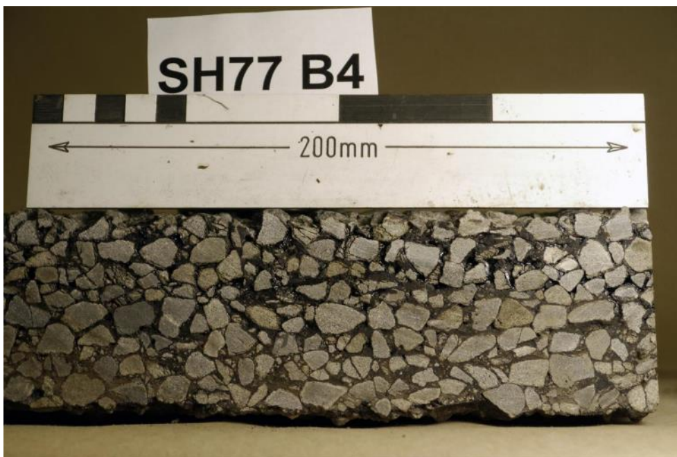
Figure 2.51 Site 4, specimen taken adjacent to the flushed patch
