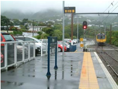
Ngaio has train indicator boards placed high up on poles (to avoid vandalism), like most stations in the Wellington region. (NJD)
