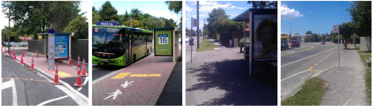
Two bus stops on Ilam Road. On the left, new pavement is being installed at a bus stop and on the right, the advertising hoarding is on the downside and does not obstruct views of buses. (JF)
