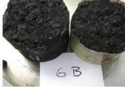
Figure 4.8 Leutner shear test blocks for T13_1404 specialist surfacing product
