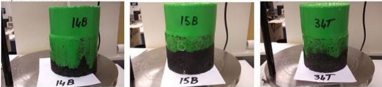
Figure 4.8 Leutner shear test blocks for T13_1403 specialist surfacing product
