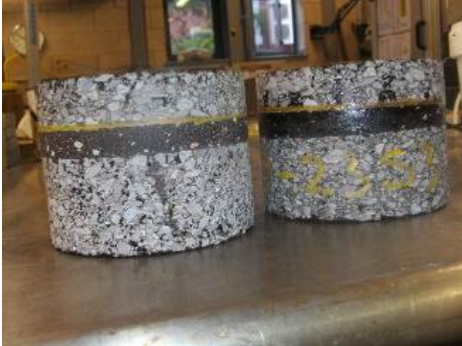
Figure 2.7 Leutner peak shear strength on cores bonded with SAMI from research at Nottingham
