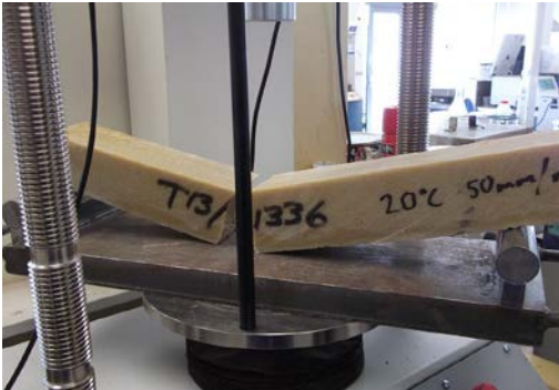
Figure 3.3a Photos of flexural beam tests on specialist resins
