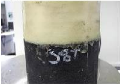
Figure 4.8 Leutner shear test blocks for T13_1404 specialist surfacing product
