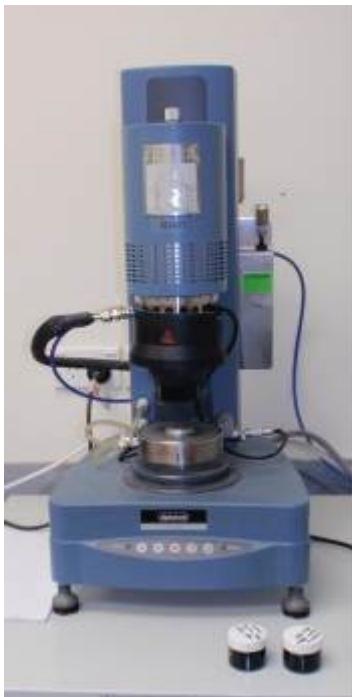
Figure 8.1 Dynamic shear rheometer test for binders
