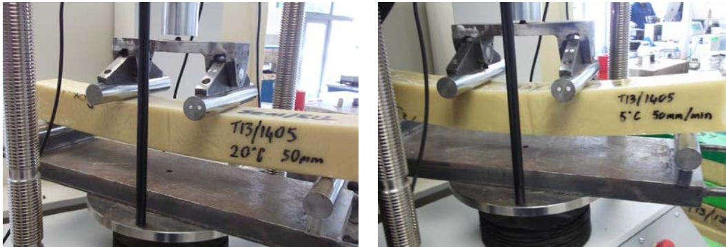
Figure 3.3b Photos of flexural beam tests on specialist resins
