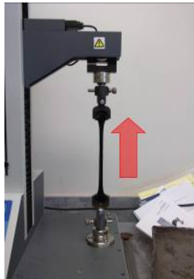
Figure 8.2 Direct tension tester for binders
