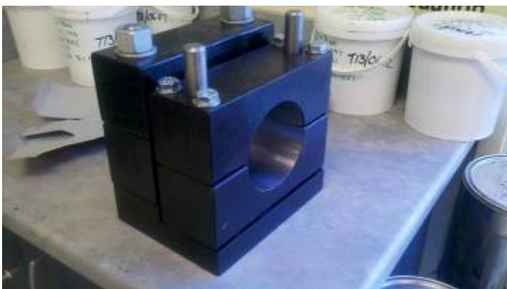
Figure 2.5 Leutner shear test apparatus
