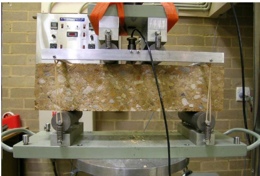
Figure 2.1 Flexural beam test
