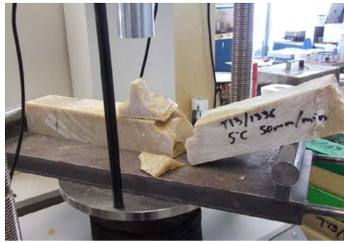
Figure 3.3a Photos of flexural beam tests on specialist resins
