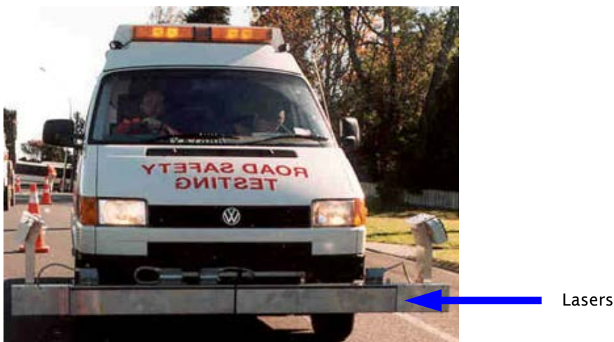
Figure 3.2 Laser profilograph owned by Pavement Management Services
