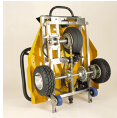
b) GripTester measuring wheel and chain transmission
