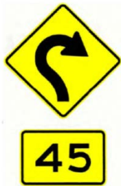
Figure 9.6 Example of a curve speed advisory sign (sourced from the NZTA Manual of traffic signs and markings 2011)
