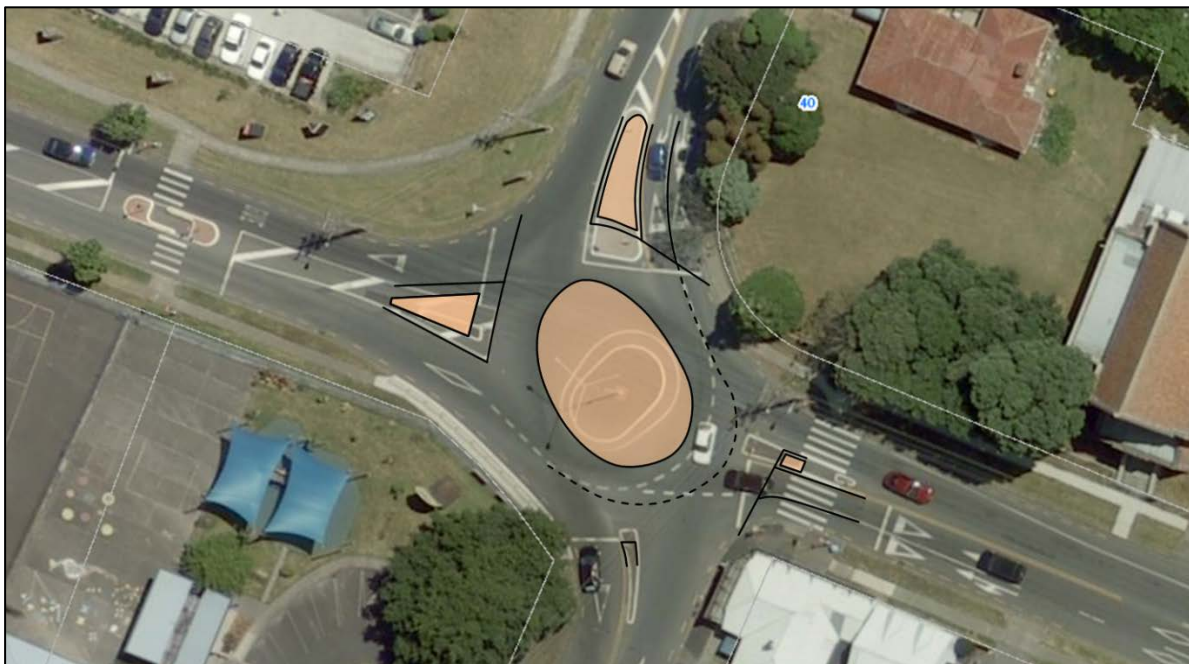
Figure 3.6 Recommended changes to Margan Ave/Hutchinson Ave roundabout to increase vehicle deflection
