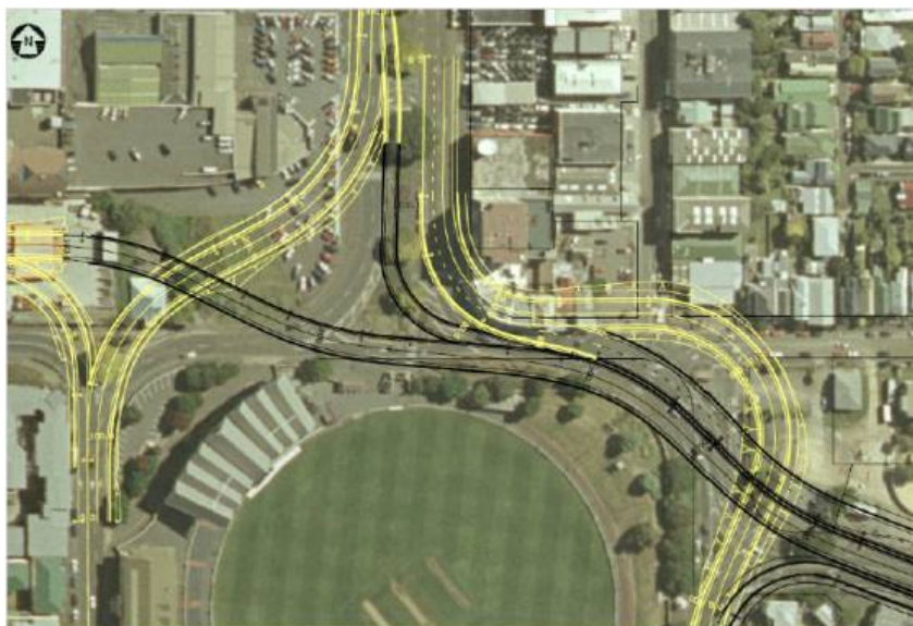
Figure F.24c Potential alignment for grade separated option at the Basin Reserve
