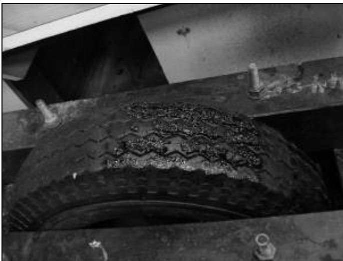
Figure 4.2 Adhesion of bitumen to the tyre
