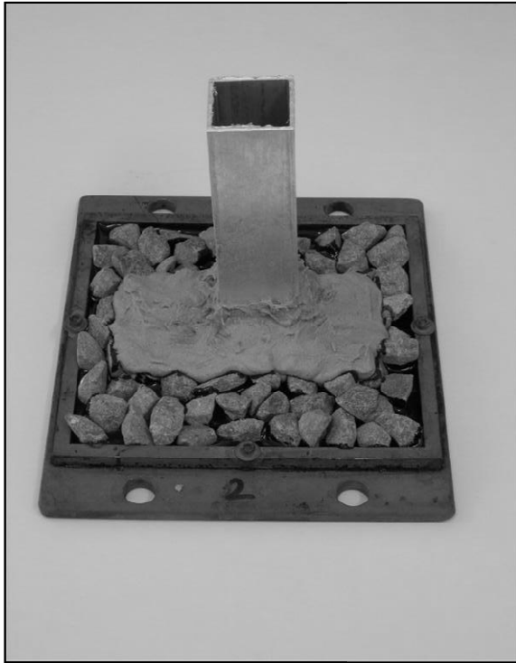
Figure 5.2 Cohesion test specimen
