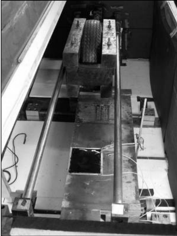
Figure 4.2 Adhesion of bitumen to the tyre
