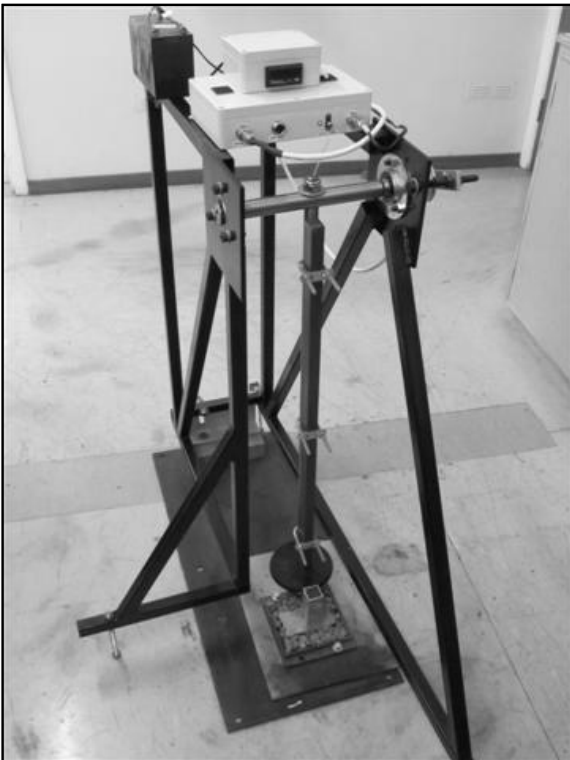
Figure 5.1 Pendulum apparatus for measuring seal cohesion (specimen in place)
