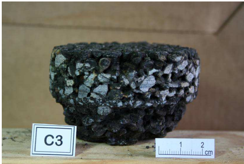
Figure 4.8 Multiple OGPA exposed to constant wet conditions in the bottom layer because of impeded side drainage (stripping of binder has occurred)
