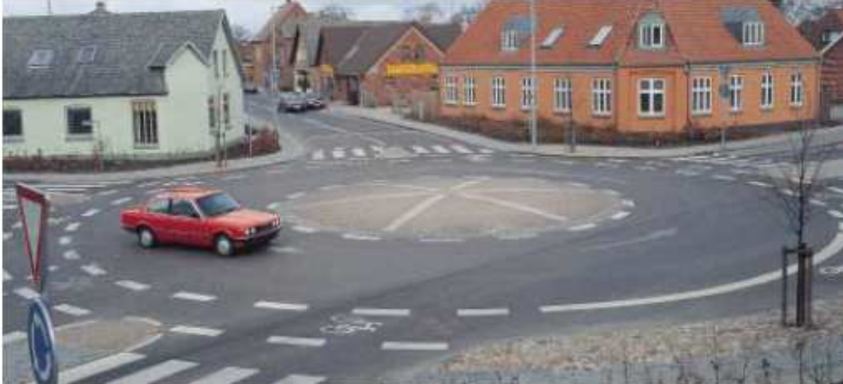
Figure 3.19 Directional cycle lanes around a roundabout in York, England (unknown source)
