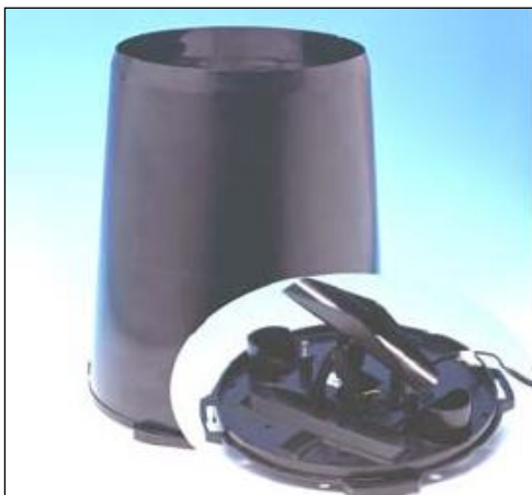
Figure 2.7 An AC013 Rain Collector showing the collection cone and a view of the interior tipping mechanism
