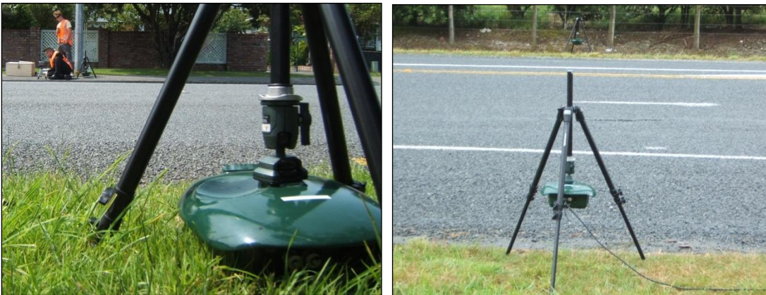
Figure 2.8 The Infrared Traffic Logger (TIRTL) roadside setup, with devices placed on opposite sides of the road to record traffic speed, headway and vehicle types
