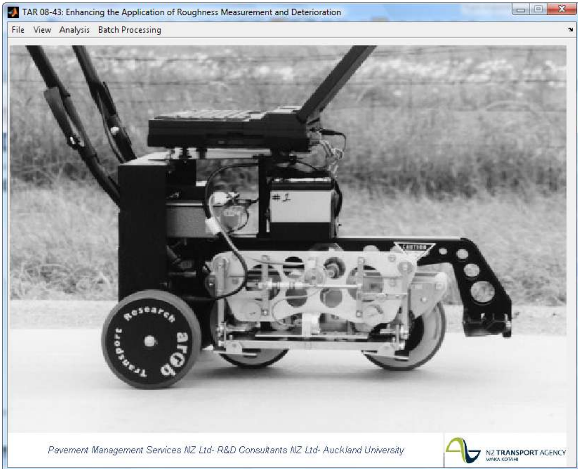
Figure B.1 Instrument used to record the pavement profile for the analysis
