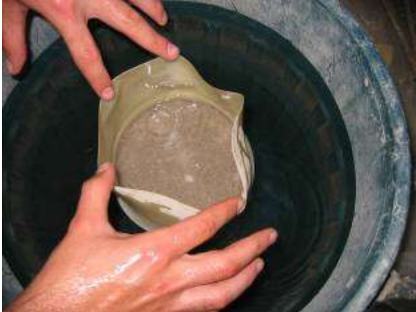
Figure 1.3 Soaking sample for a saturated undrained RLT test
