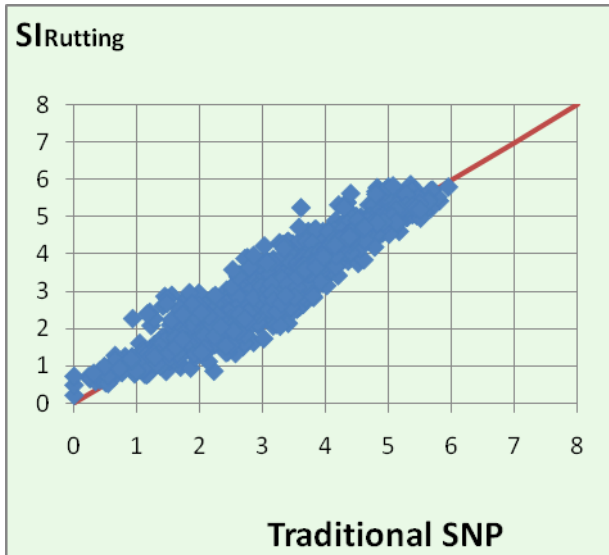
Figure 3.3 SI_{Rutting} vs SNP for LTPP site data
