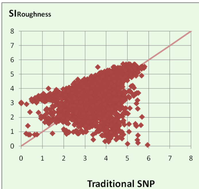
Figure 3.5 SI_{\text{Roughness}} vs SNP for LTPP site data
