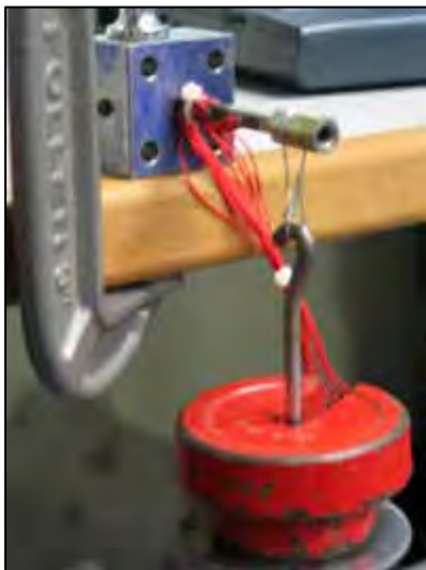
Figure 3.3 Calibration of strain-gauged pin
