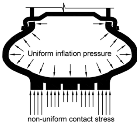
Figure 2.1 Cross section of tyre with low inflation pressure under heavy load (after Lippmann (1985))
