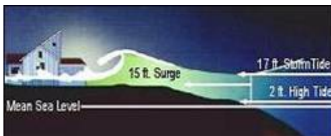
Figure 8.4 Effects of storm surge.
