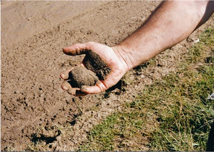
Figure 3.12 Hand squeezing method to establish optimum moisture content.
