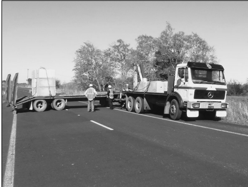
Figure 3.2 The test vehicle jack-knifed into position ready to be driven forward and the towing force measured in the thirteen tonne experiment.
