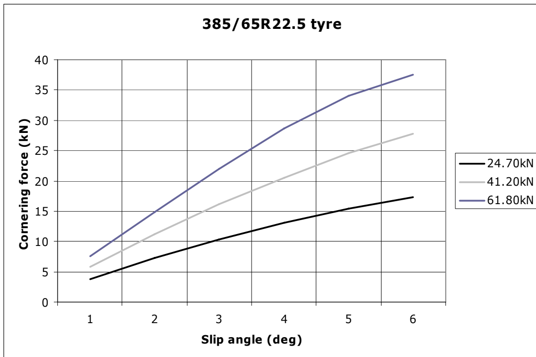
Figure 2.1 Relationship between cornering force and slip angle by vertical load for 385/65R22.5 tyres (taken from tyre manufacturers' data sheets and unpublished data from the University of Michigan Transportation Institute).
