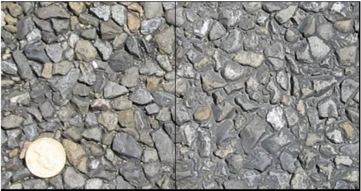
Figure A2 Watercut surface left of line and untreated 16-year-old chipseal right.
