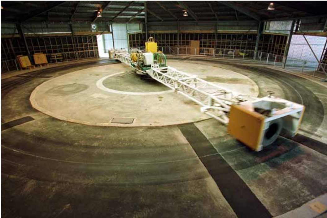
Figure 4.1 Transit New Zealand's pavement testing facility CAPTIF.
