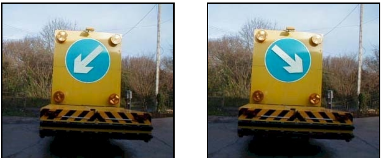
Figure 6.5 Standard TMA used in the UK, the arrow board of which can be changed (from the driver's cabin) to show different directions.
