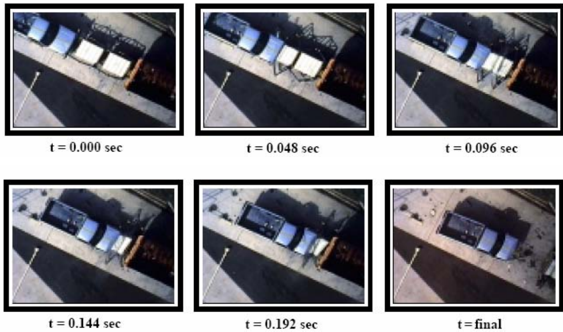
Figure 4.2 Safe-Stop 180 kph Crash Cushion impact (Griffith 2003).
