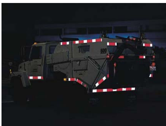
Figure 4.1 Identifying maintenance vehicles using retroreflective tape.
