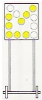
Figure 6.15 Advance warning with skewed arrow panel used on a German road if visibility is less than 400 m, as for Scenario 3.
