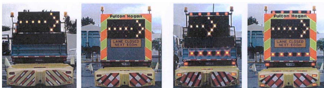
original set-up for high intensity traffic 'Smartstop' stoplights combination of all Figure 5.1 Some improvements made to the visual appearance of TMA.
