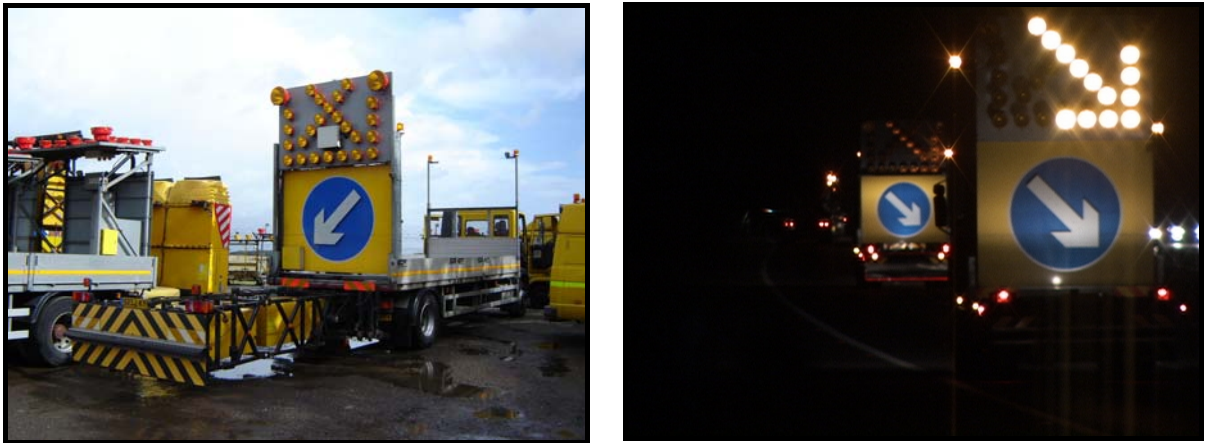
Figure 6.6 TMA with Skew Arrow Board, used in the UK for risky operations at night or in heavy traffic.
