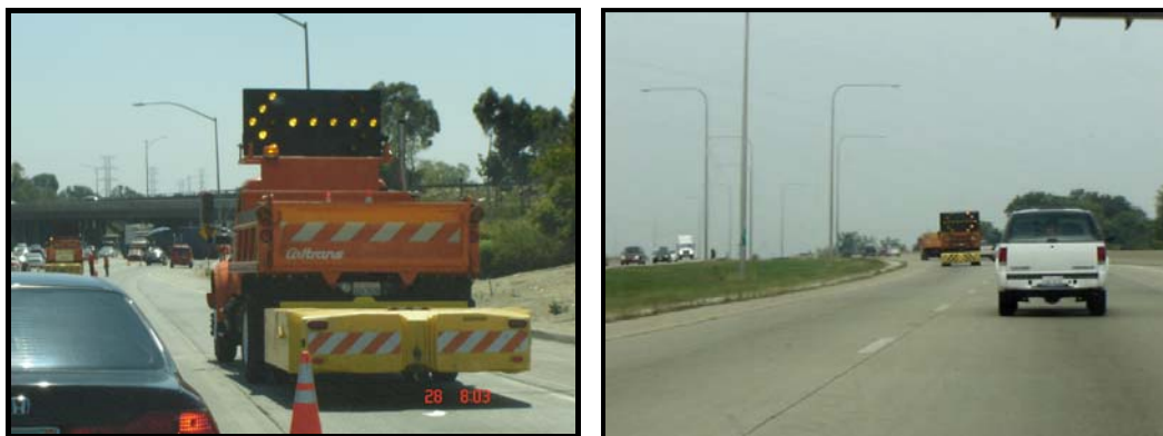
Figure 6.1 Typical TMA used in the US. Appearance when viewed close up (left) and from a distance (right).
