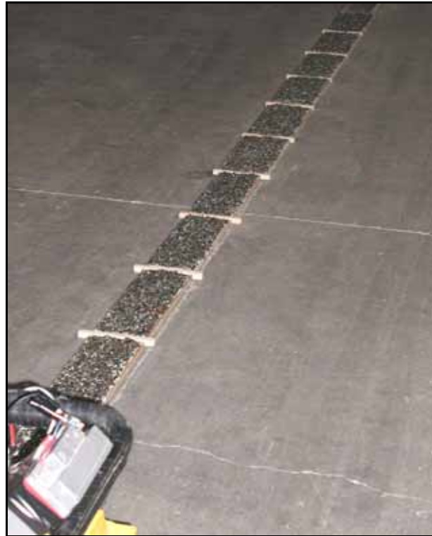
Figure 8.2 Test plates showing wooden-inserts to reduce GripTester 'bounce'.
