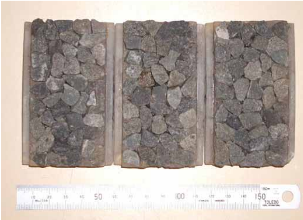
Figure A3.3 PSV' samples, Pound Road quarry, sealing chip.
