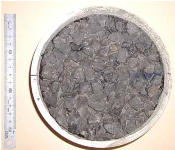
Figure A4.12 Hastings Quarry aggregate, grade 3, between wheelpaths, 'high' HCV passes (direction of traffic = ↔).
