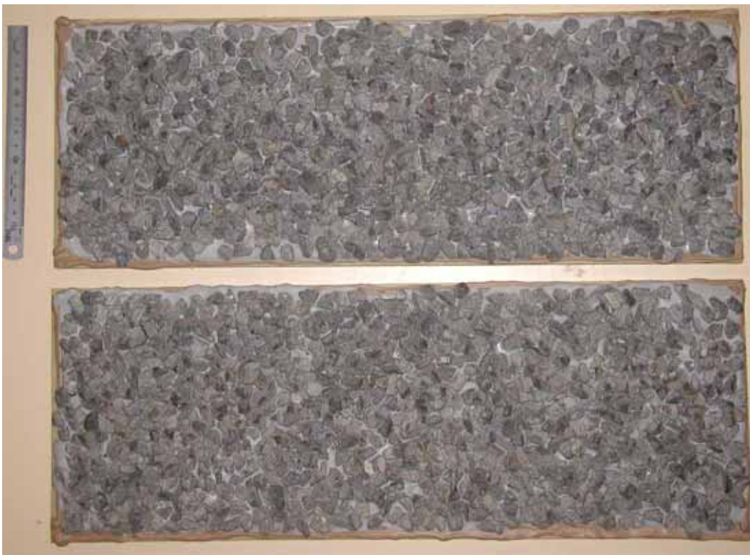
Figure A2.2 70% crushed (top) and 80% crushed (bottom), Pound Road quarry, pass 13.2 mm, held 9.5 mm.
