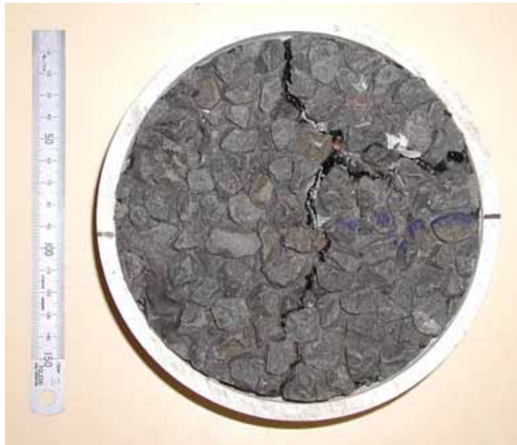
Figure A4.7 Hastings Quarry aggregate, grade 3, left wheelpath, 'low' HCV vehicle passes (direction of traffic = ↔).
