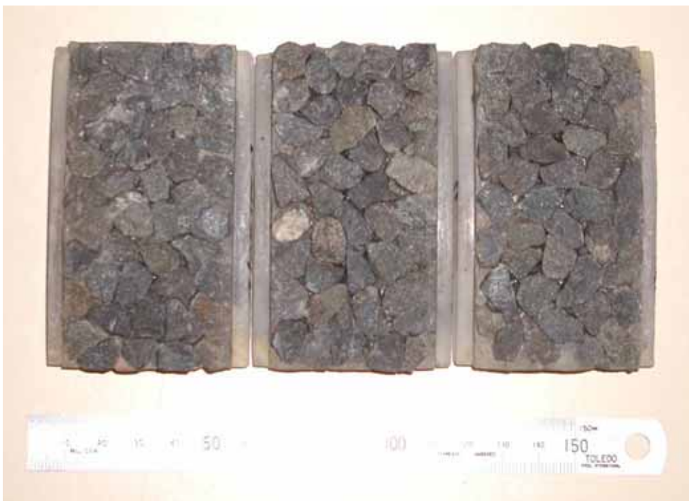
Figure A3.4 PSV' samples, Hastings quarry, sealing chip.
