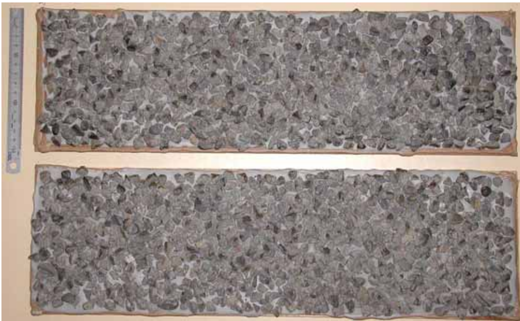
Figure A2.5 80% crushed (top) and 90% crushed (bottom), Hastings quarry, pass 13.2 mm, held 9.5 mm.
