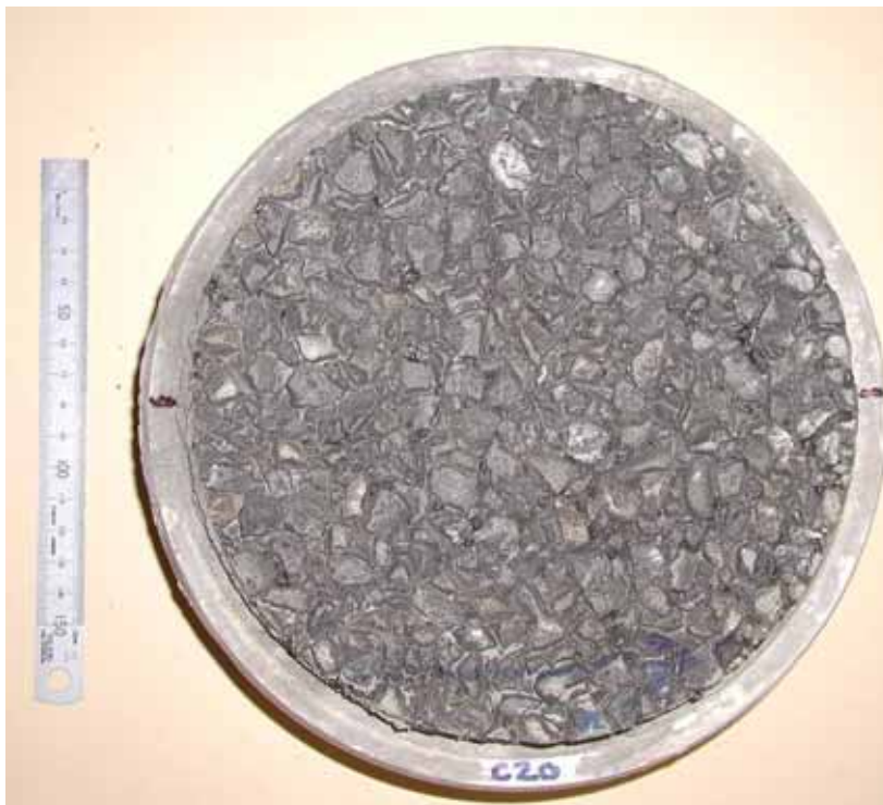
Figure A4.1 Pound Road aggregate, grade 3, left wheelpath, 'low' HCV passes (direction of traffic = ↔).
