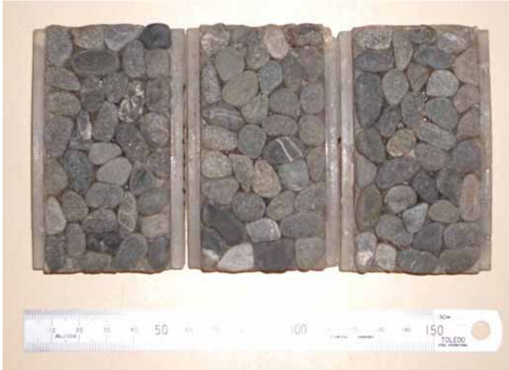
Figure A3.1 PSV' samples, Pound Road quarry, pea-gravel.
