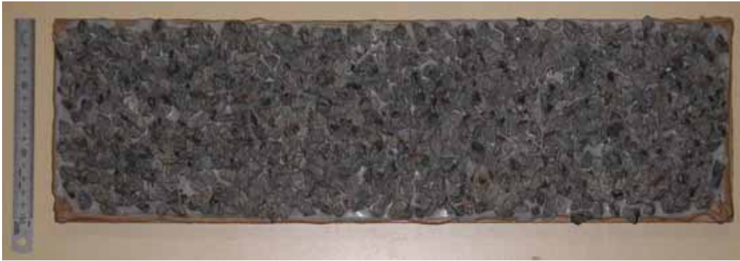
Figure A2.6 100% crushed, Hastings quarry, pass 13.2 mm, held 9.5 mm.
