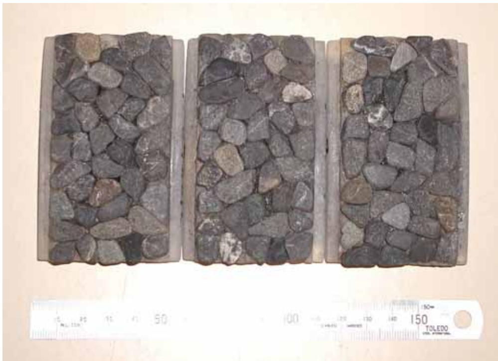
Figure A3.1 PSV' samples, Pound Road quarry, pea-gravel.
