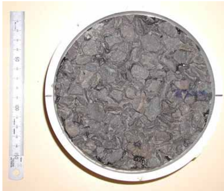
Figure A4.9 Hastings Quarry aggregate, grade 3, left wheelpath, 'high' HCV passes (direction of traffic = ↔).
