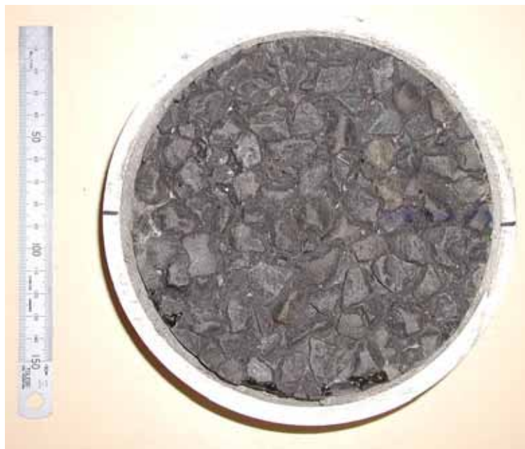
Figure A4.8 Hastings Quarry aggregate, grade 3, left wheelpath, 'medium' HCV vehicle passes (direction of traffic = ↔).
