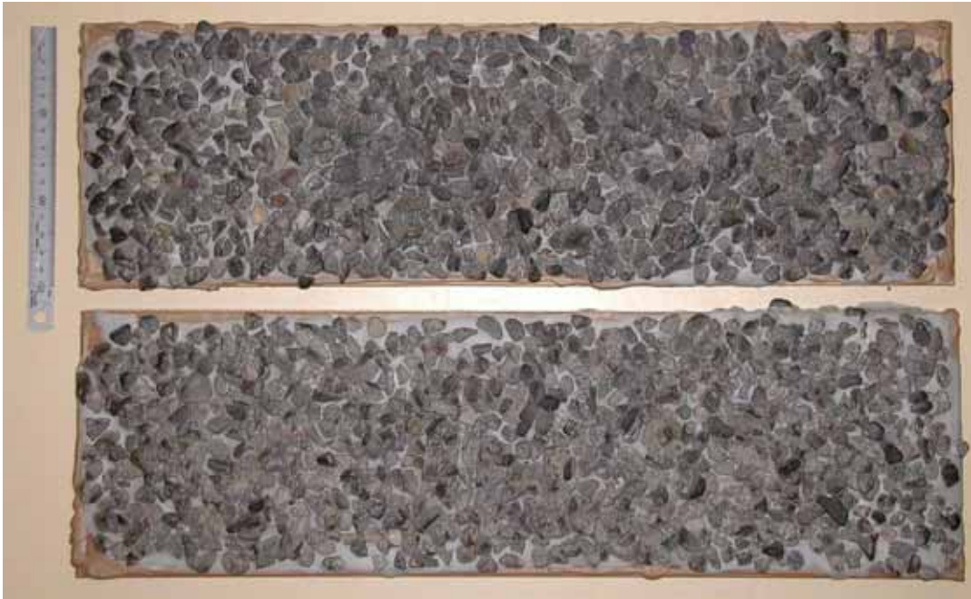
Figure A2.4 0% crushed (top) and 50% crushed (bottom), Hastings quarry, pass 13.2 mm, held 9.5 mm.
