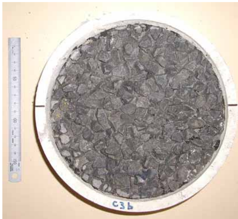
Figure A4.6 Pound Road aggregate, grade 3, between wheelpaths, 'high' HCV Passes (direction of traffic = ↔).
