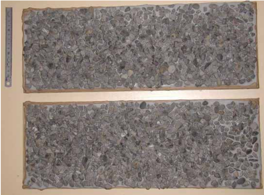
Figure A2.2 70% crushed (top) and 80% crushed (bottom), Pound Road quarry, pass 13.2 mm, held 9.5 mm.
