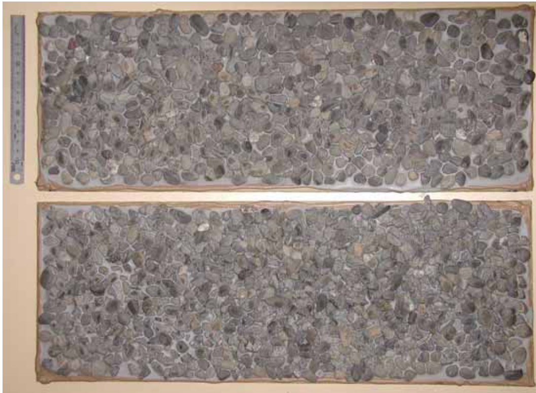
Figure A2.1 0% crushed (top) and 50% crushed (bottom), Pound Road quarry, pass 13.2 mm, held 9.5 mm.
