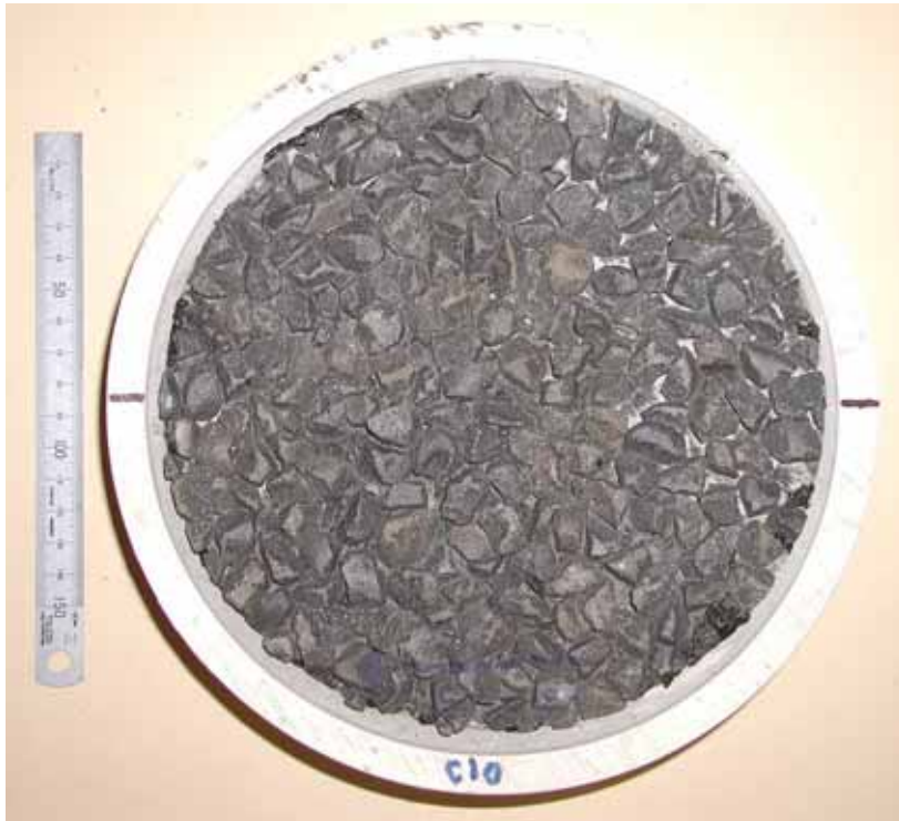
Figure A4.1 Pound Road aggregate, grade 3, left wheelpath, 'low' HCV passes (direction of traffic = ↔).
