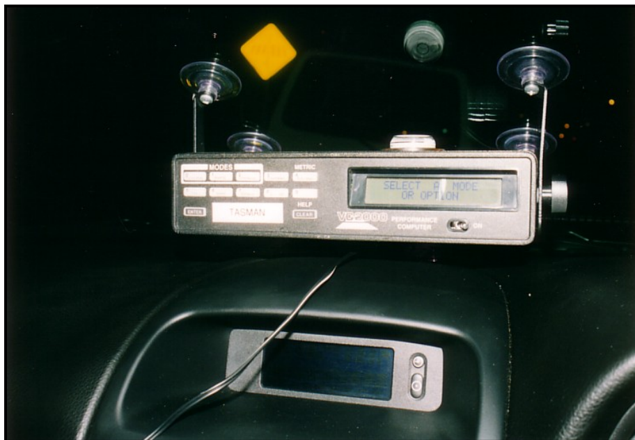
Figure 4.3 Vericom VC2000 unit mounted on the windshield of the test vehicle.
