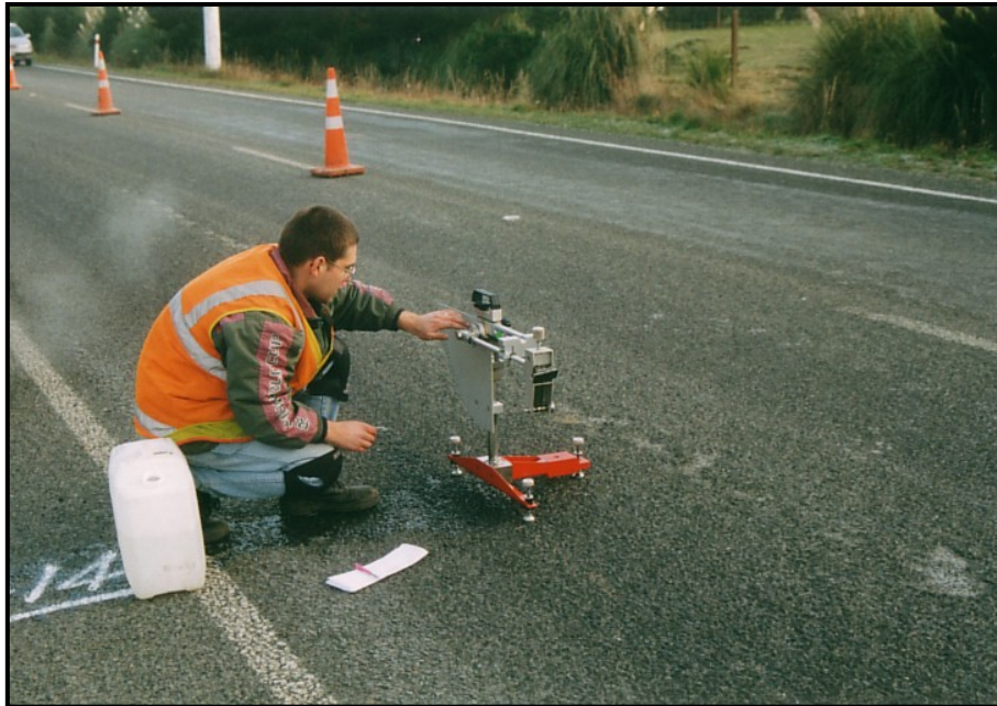
Figure 4.1 British Pendulum Tester in use on one of the test sites.
