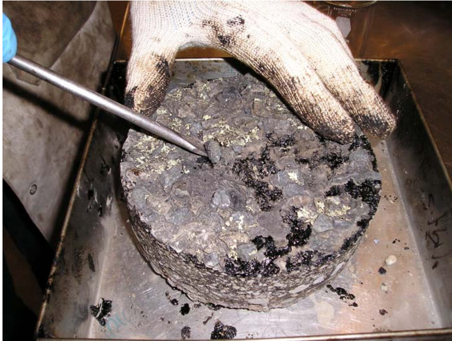
Figure 2.4 Removal of chips for bitumen extraction.
