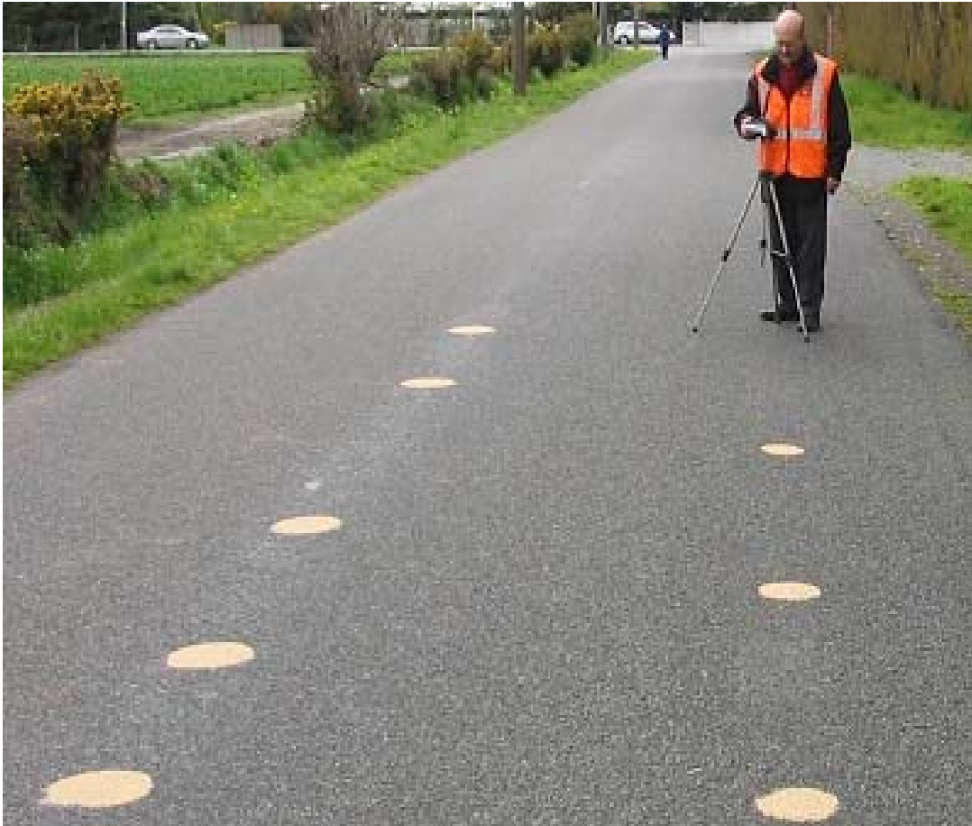
Figure 3.3 Sand circle testing protocol.
