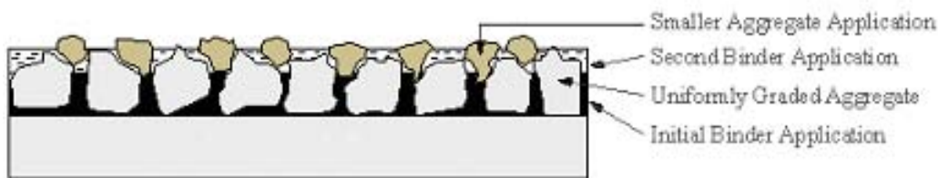
Figure 2.3 Double chipseal.
