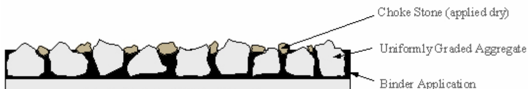
Figure 2.4 Racked-in seal.
