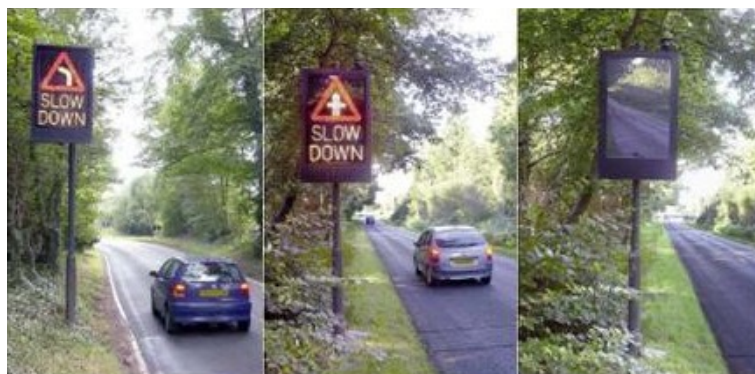
Figure 2.1 Vehicle-activated VMS warnings (left to right) curve warning, crossroads warning, and VMS in the 'Off' state (from Winnett & Wheeler 2002).
