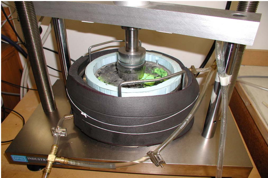
Figure 3.1 Sample mounted for testing, with insulating polystyrene sheet removed to show the seal surface.
