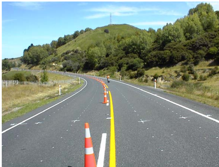
Figure 3.4 Example of a Transit New Zealand calibration section.
