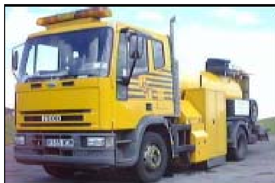
Figure 2.3 WDM SCRIM (sideways force coefficient routine investigation machine) and survey vehicle.
