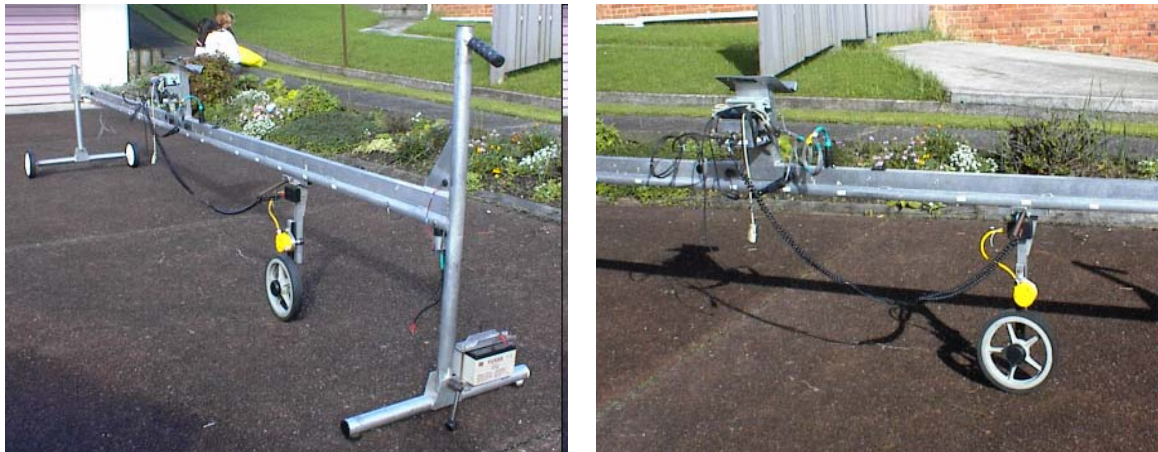
Figure 3.1 DCL Transverse Profile Beam.
