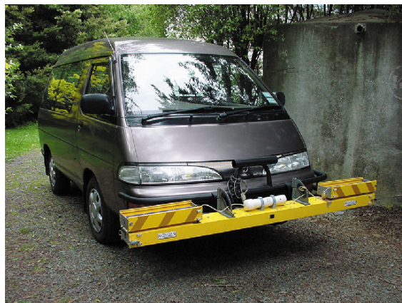
Figure 2.2 MWH ROMDAS ultrasonic profilometer.
